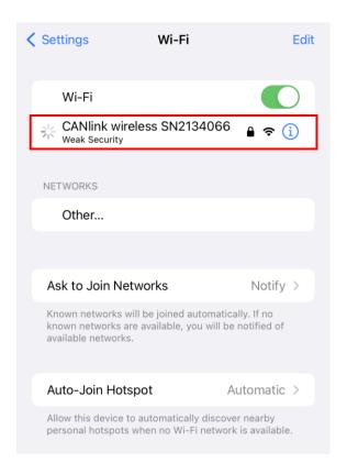
It is very important to wait for the connection to the Wi-Fi network to be established correctly. When the connection stage is complete, a blue validation icon appears, as shown below:
